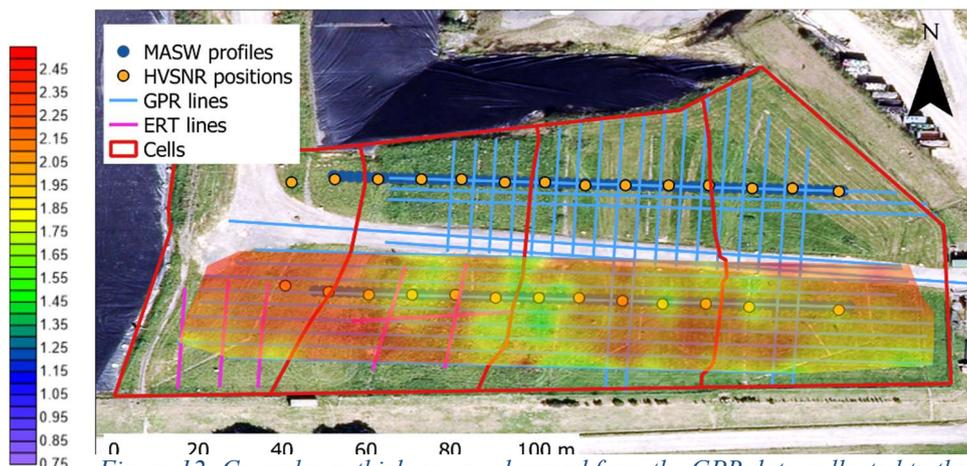
*Figure 12: Cover layer thickness as observed from the GPR data collected to the South of the access road. This data was extrapolated to construct the upper waste boundary of the RDM.*
