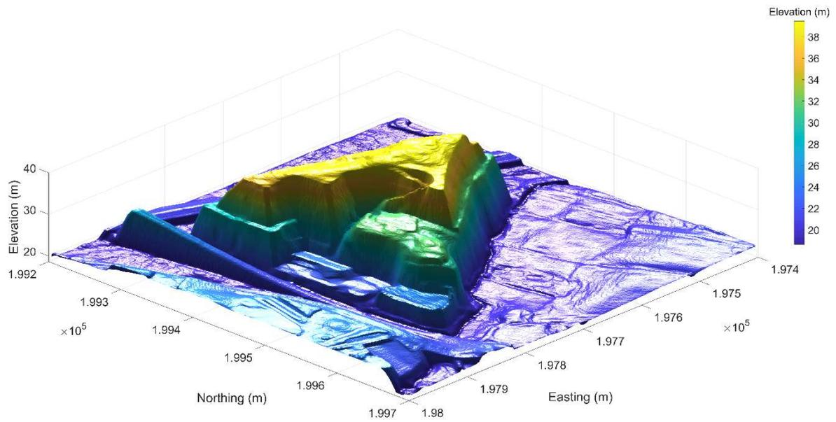
Figure 9: Digital Elevation Model (DEM) of the Meerhout landfill obtained from LIDAR data (vertical view exaggerated).
