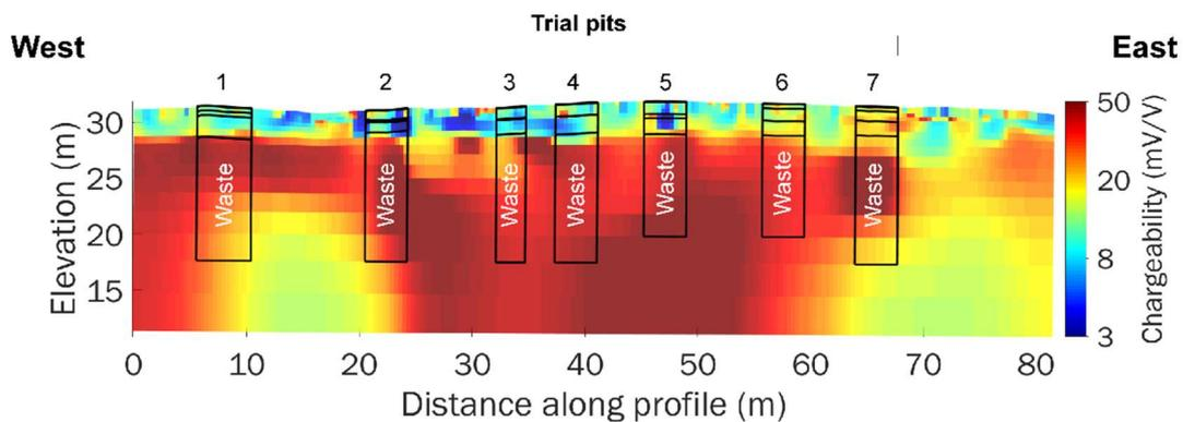
Figure 6: High-resolution chargeability profile obtained just before the last phase of the sampling (trial pitting). The high chargeability corresponds to the main waste body.
