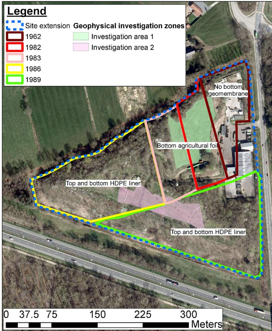
Figure 1: The Meerhout landfill installation with successive development phases of the site.
