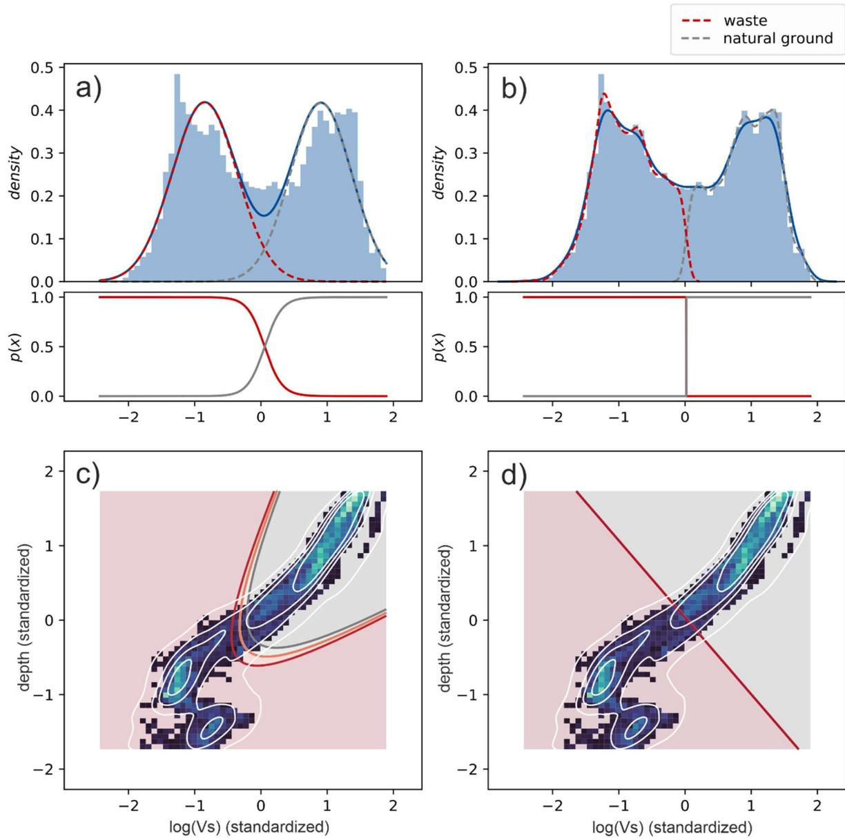
Figure 13: Comparison of different clustering approaches to categorise the MASW data into waste and natural ground. The conditional probabilities in a & c were derived by using a Gaussian mixture model. b & d were derived by KMeans clustering. In c & d, the depth was included as an additional attribute.
