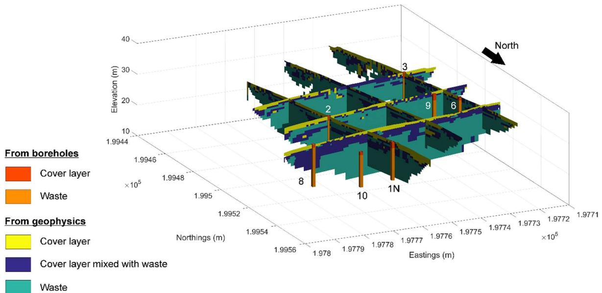
*Figure 8: RDM in the lower zone: the waste body is represented in green, yellow is the cover layer and blue is the cover layer material mixed with waste. Boreholes are the bars where red is the cover layer found and orange the waste extension.*
