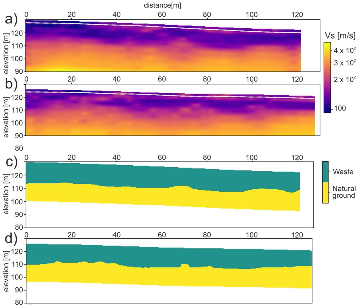
Figure 14: a & b) Shear wave velocity of the two West-East aligned MASW profiles. c & b) Delineation of the waste material derived by KMeans clustering including the shear wave velocities as well as the depth of the two profiles in a & b. It should be noted that the cover layer thickness indicated by the white line in a & b as well as the lateral cell boundaries could not be resolved with the MASW data.
