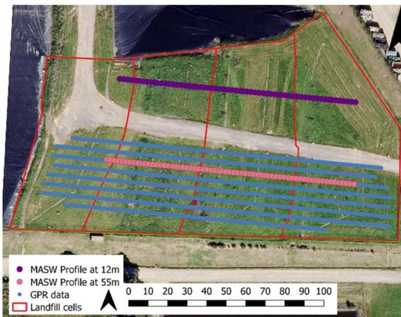
*Figure 11: Extent of the geophysical data (MASW and GPR) to create the RDM*
