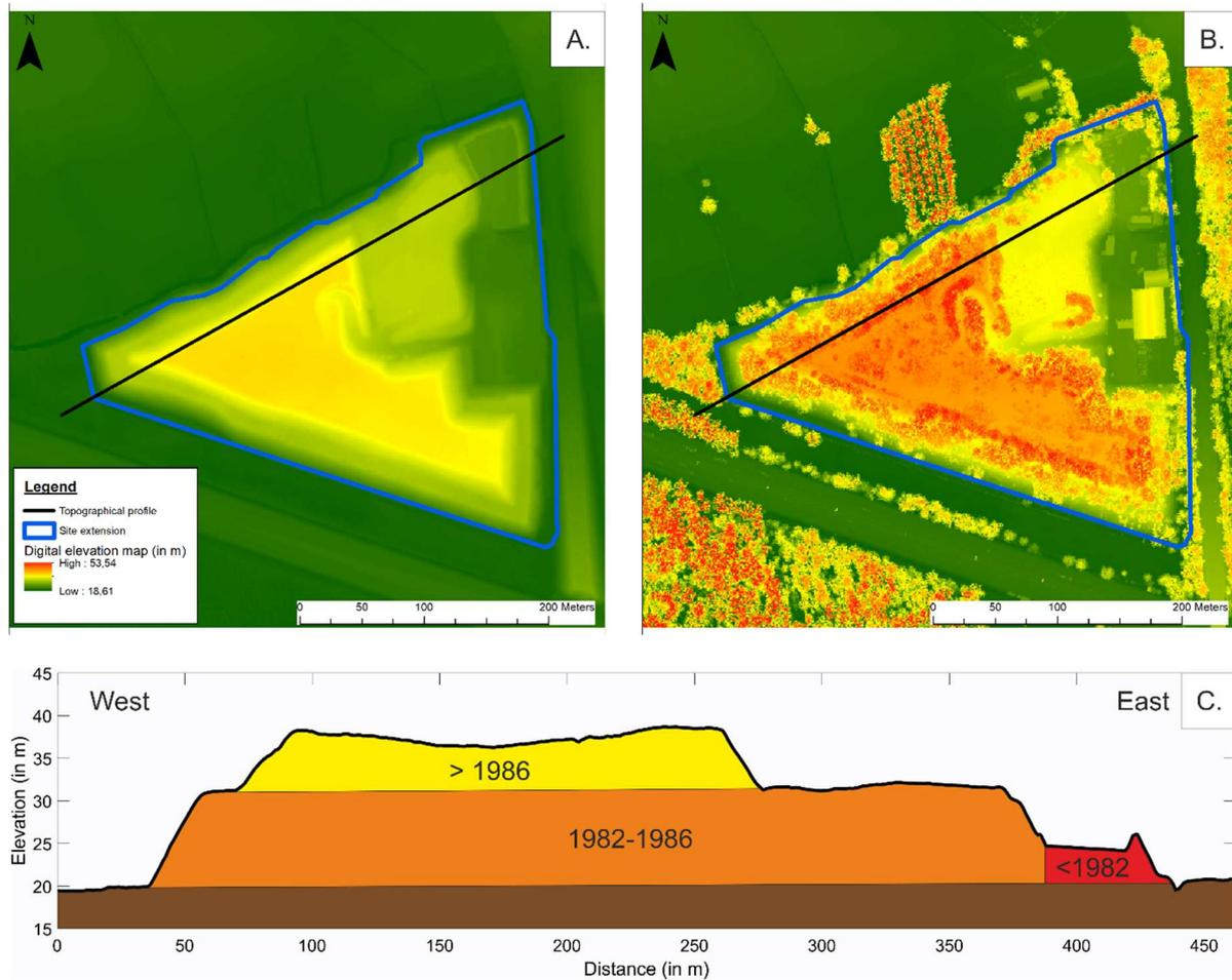
Figure 2: The Meerhout landfill topography: A. DEM soil elevation; B. DEM top of vegetation; C. cross-section
