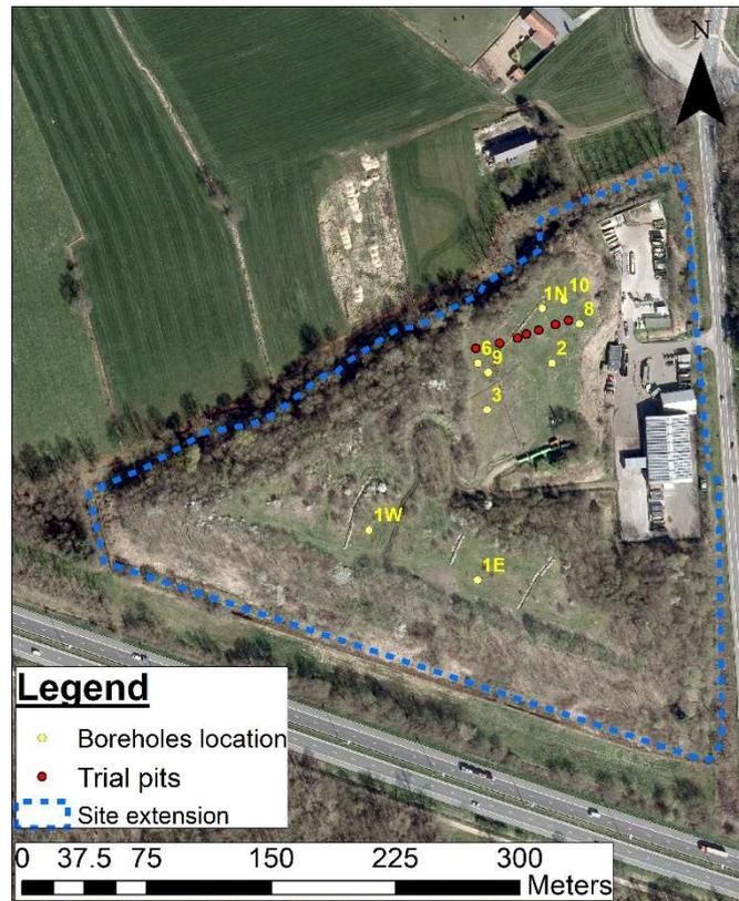
*Figure 4: Sampling carried out in Meerhout consisting in 9 boreholes and 7 trial pits.*
