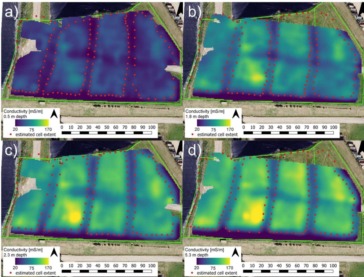
Figure 15: a to d) Conductivity maps derived from the EM measurements. The EM data was used to estimate the lateral extent of the waste cells as indicated with red dots.
