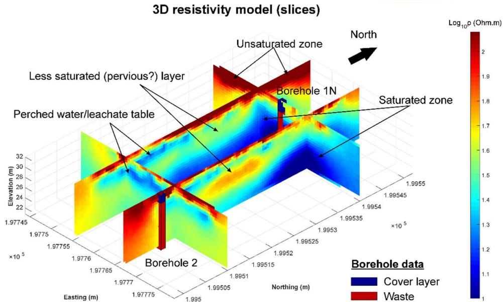
Figure 5: Electrical resistivity transects extracted from the 3D ERT model
