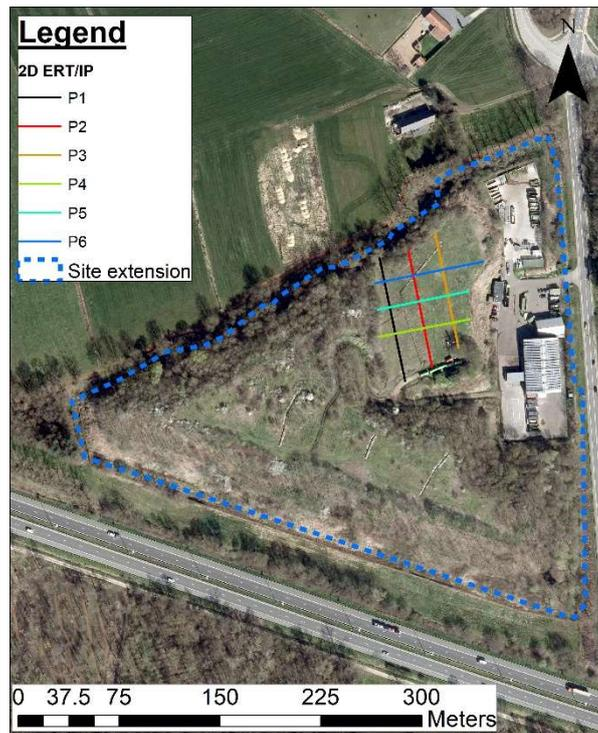
*Figure 7: ERT and IP profiles used to derive the RDM in the lower zone of the landfill.*
