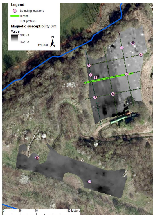
Figure 12: Magnetic susceptibility map derived from the in-phase data measured with the 2 m antenna and horizontal coil alignment. Investigation depth is 3.0 m.
