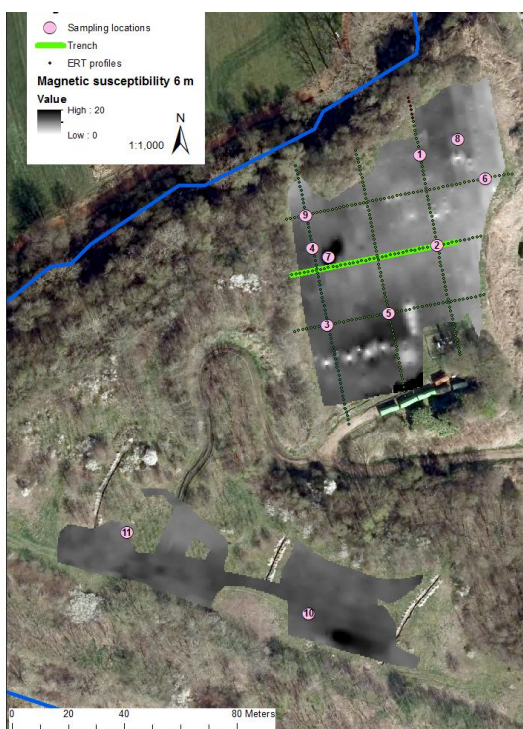
Figure 13: Magnetic susceptibility map derived from the in-phase data measured with the 4 m antenna and horizontal coil alignment. Investigation depth is 6.0 m.
