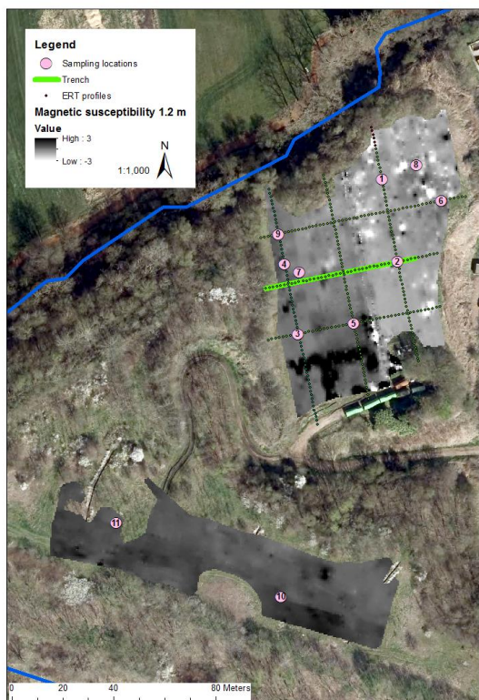
Figure 10: Magnetic susceptibility map derived from the in-phase data measured with the 2 m antenna and vertical coil alignment. Investigation depth is 1.2 m.
