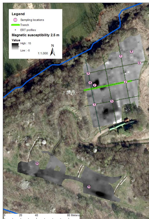
Figure 11: Magnetic susceptibility map derived from the in-phase data measured with the 4 m antenna and vertical coil alignment. Investigation depth is 2.5 m.
